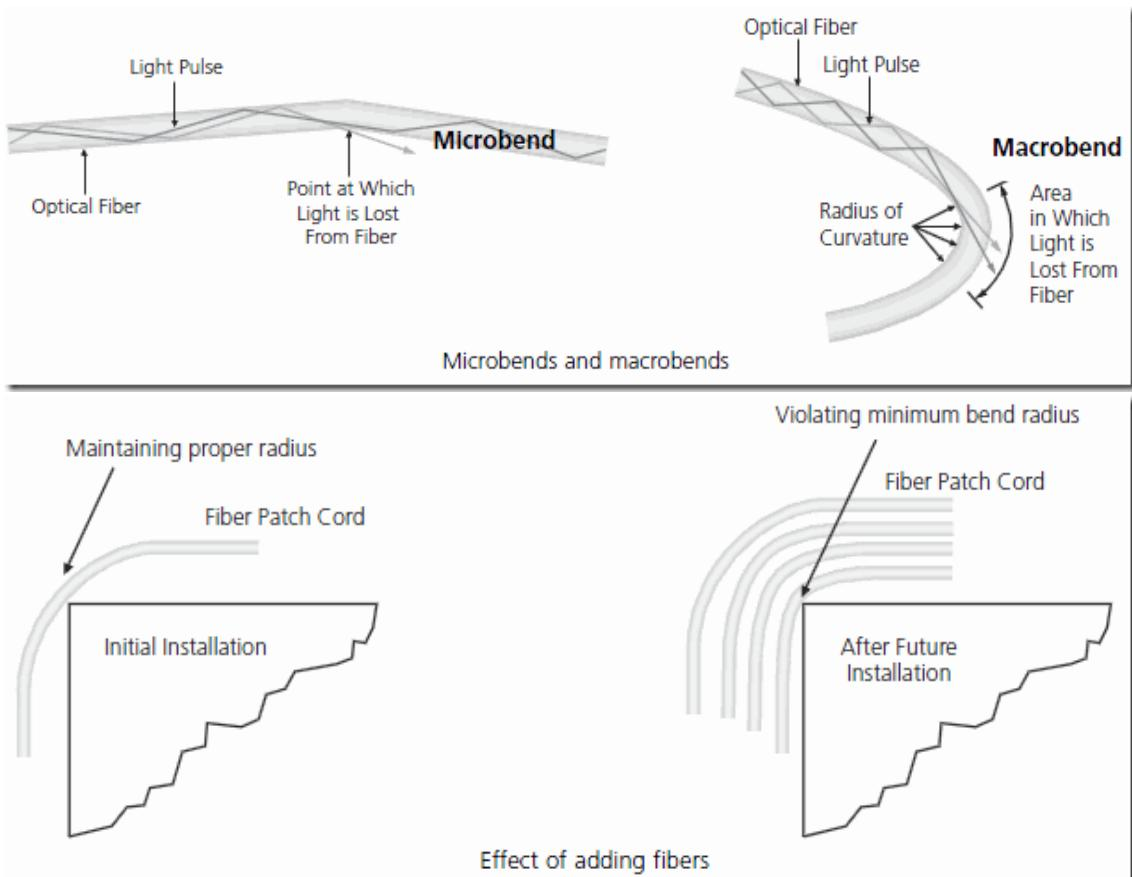
in general, the minimum bend radius should not be less than ten times the outer diameter (OD) of the fiber cable. Thus a 3mm cable should not have any bends less than 30mm in radius.
