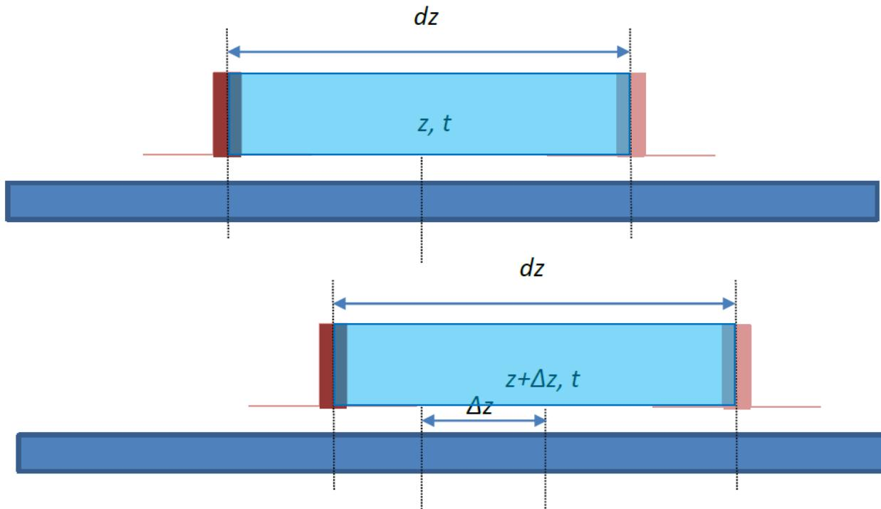
Illustration of two spatially-consecutive iDAS measurements, at  $z, t$  and  $z + \Delta z, t$ .  $dz$  is the gauge length, which is generally larger than the sampling resolution,  $\Delta z$ , the distance between consecutive measurement points
