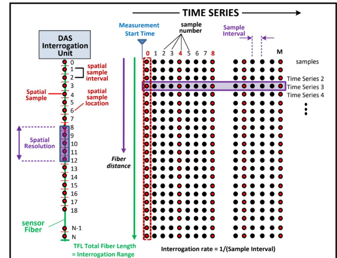
Figure 3. Signal Parameters relating to Time Series and their Spatial Location Identification
