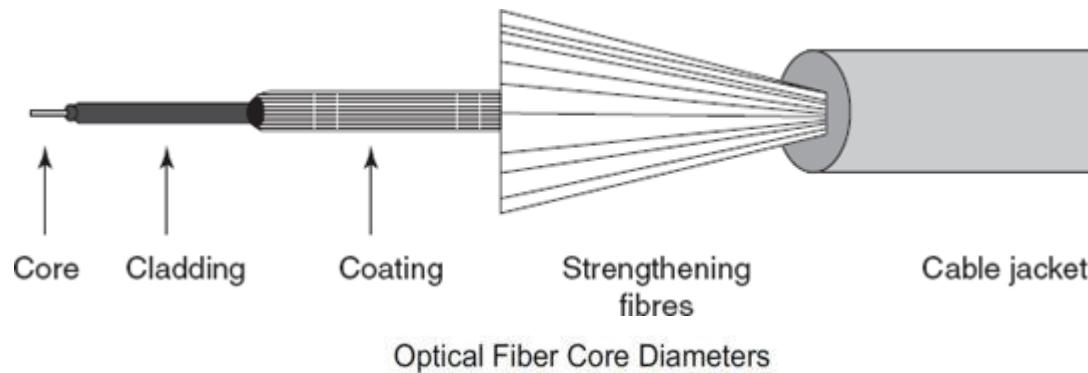
Optical Fiber Core Diameters
