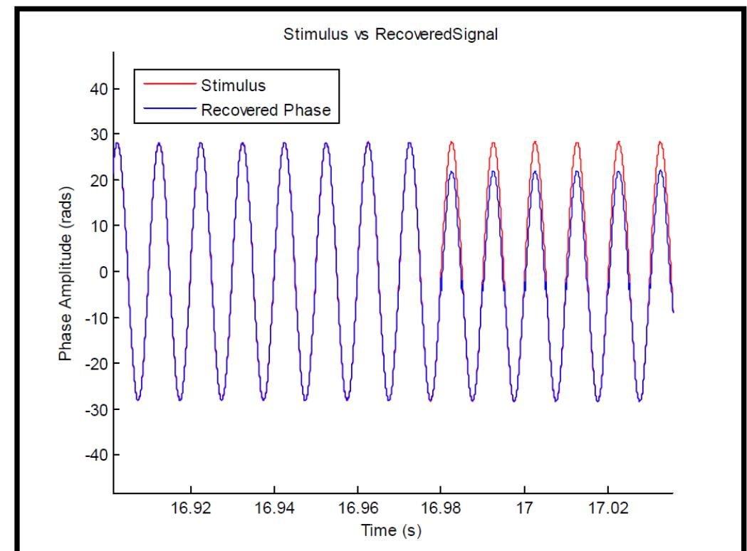
Figure 21. Zoom view of stimulus signal and IU response showing phase jump at 16.98 seconds
