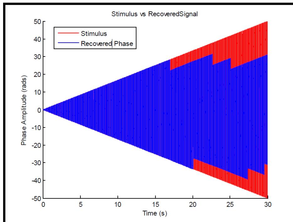
Figure 20. Stimulus signal (red) and IU response (blue) showing linear limit at 17 seconds
