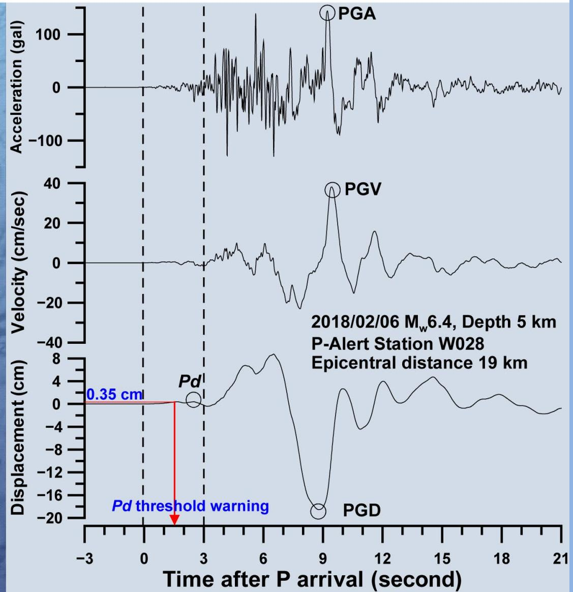
Combination with modern MEMS sensor. Cheaper device may install to every building to give warning within three seconds after P arrival after a large earthquake occurs.
